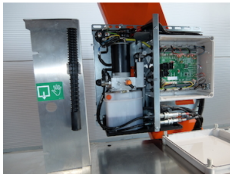
Hydraulic pump unit 12V or 24V DC, including emergency functions
