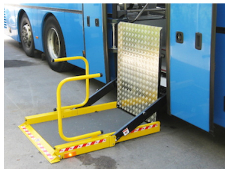
OWP005 - Non-standard length of the bridge plate
