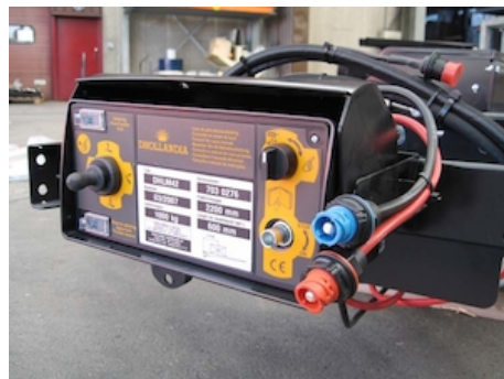
OAE506 - CANNON plug for connection 25mm² cable
