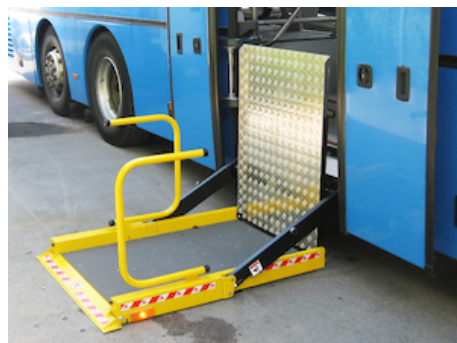
OWP005 - Non-standard length of the bridge plate
