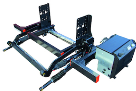
OAT102 - Standard finish of lift frame: KTL + powder coat
