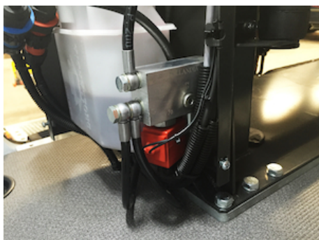
OWH001 - Flow regulator open / close on DH-PH2/P2
