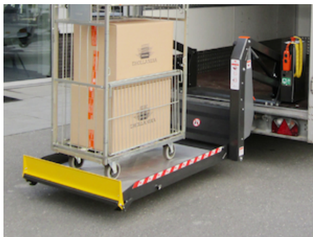
Automatic roll-stop at the outboard platform edge
