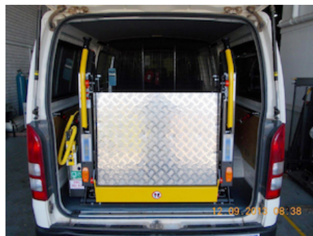
OWU003 - Horizontally folding platform DH-PH2/P2
