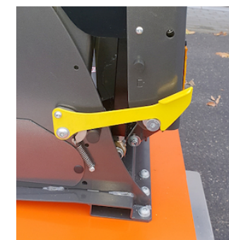
OWF015 - Lock PH2 with spring instead of gas pump
