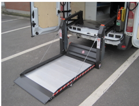
750 kg execution: platform reinforced by steel cable suspension
