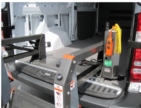
12V or 24V DC pump unit premounted at the side of the lift frame
