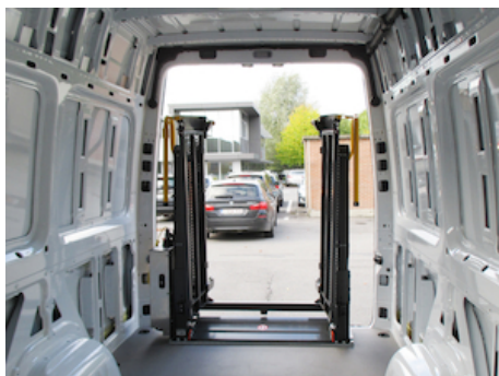
OWU002 - Vertically folding split platform DH-PH2/P2 type2
