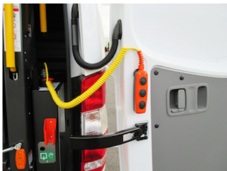
OWE002 - 3-button wander lead + limit switch on lift movement
