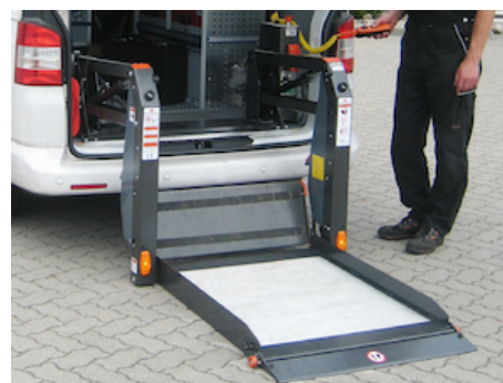
OWP001 - Bridge plate mounted on inboard platform edge
