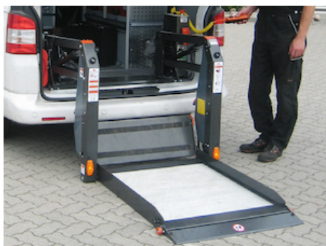
OWP001 - Bridge plate mounted on inboard platform edge
