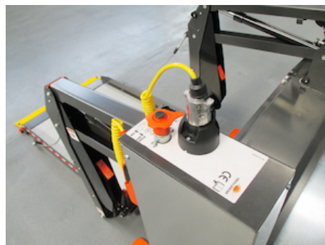
OWE004 - Plug connection for wander lead on pump unit
