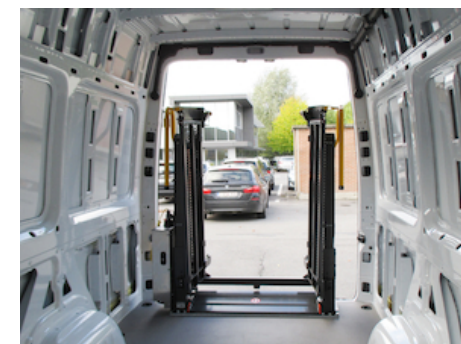
OWU002 - Vertically folding split platform DH-PH2/P2 type2
