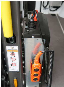
12V or 24V DC pump unit premounted at the side of the lift frame
