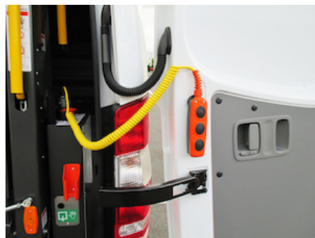
OWE002 - 3-button wand lead + limit switch on lift movement
