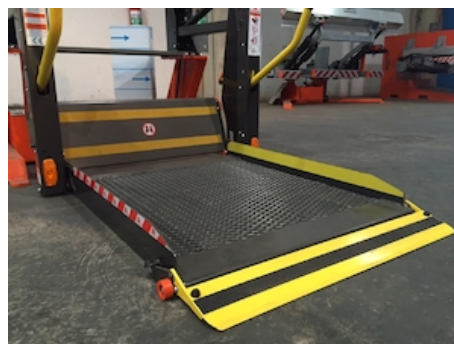
OWP004 - Yellow signalisation on DH-P platform
