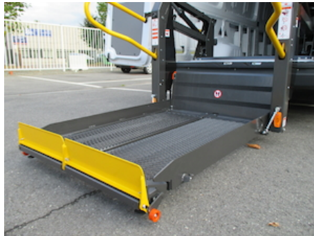
Automatic roll-stop at the outboard platform edge
