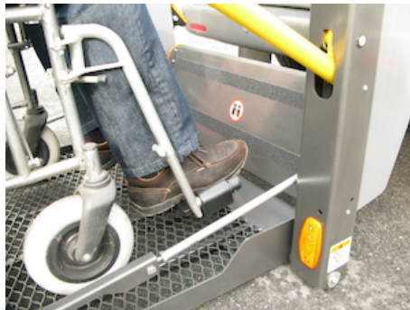
Automatic bridge plate + toe-guard + load restraint at the inboard platform edge
