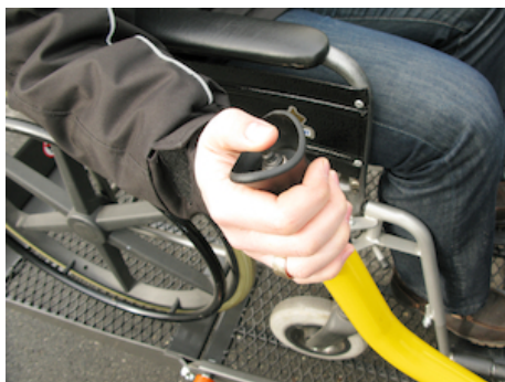
OWE001 - Toggle switch up / down on safety rail
