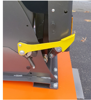
OWF015 - Lock PH2 with spring instead of gas pump
