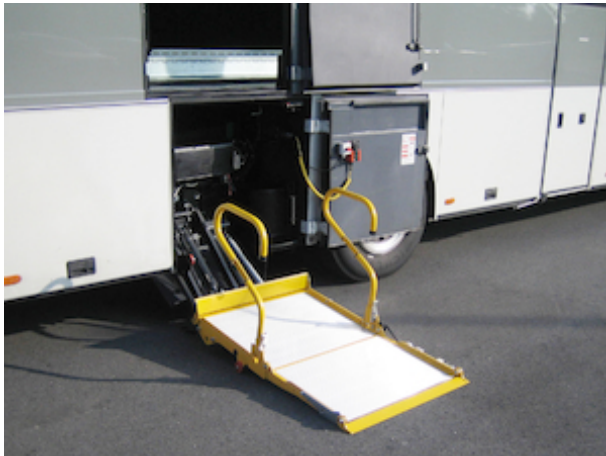
DH-RB unfolded in work position [+ option OWP011]
