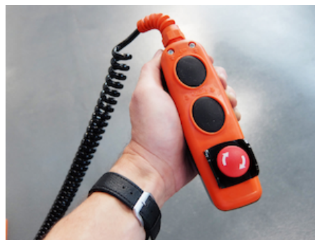
OWE005.02 - Emergency stop integrated in wander lead
