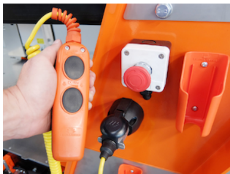
OWE005.01 - Emergency stop in separate box
