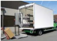
In its travel position, the interior lift **DH-VZS** is stowed against the side of the body and offers the driver **quick and free access** through the vehicle doors. Upon use, the platform is simply pulled out and opened by hand. As the platform slides straight towards the door exit, the floor space beside it can be fully occupied by cargo (as opposed to the DH-VZ.03). A wander lead with spiral cable is used to operate the platform up and down.
