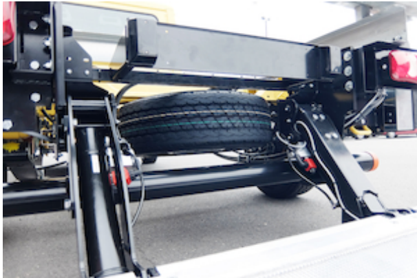
The lift frame without cross tube enables to keep the spare wheel in its original position in most cases
