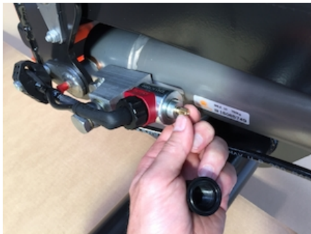
Manual emergency operation on all electrovalves
