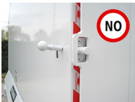
OAP420 - DH-L* platform without lock (on client's request)
