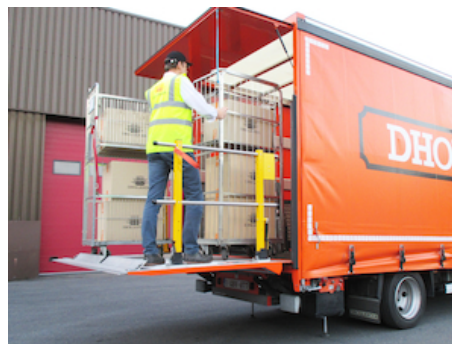
OAP202.LR - 2 hinged safety rails on L+R side of platform
