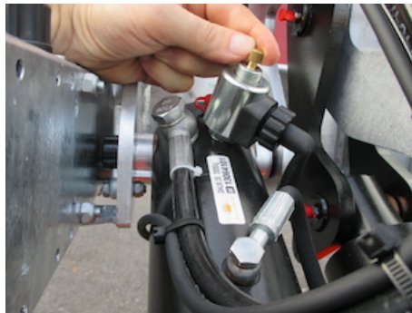
Manual emergency operation on all electrovalves
