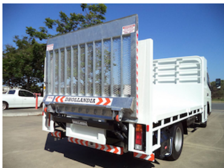
OAP018.01 - Platform of DH-L* in wind-permeable meshed steel
