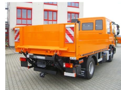
OAP403.1 - Horizontally folding point on DH-L* platform, full width
