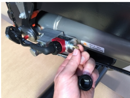
Manual emergency operation on all electrovalves
