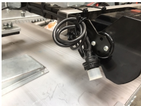
OAE500 - VEHH plug connection for dashboard switch
