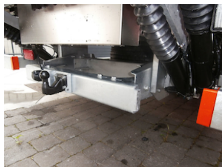
OAF103 - Suppl. for preparation of the bumper bar for towing hitch
