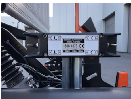
OAE048.0 - Control unit with 2 toggle-switches
