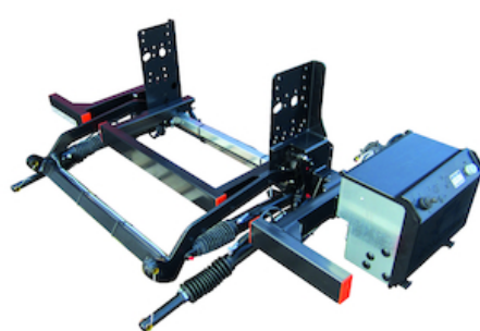
OAT102 - Standard finish of lift frame: KTL + powder coat
