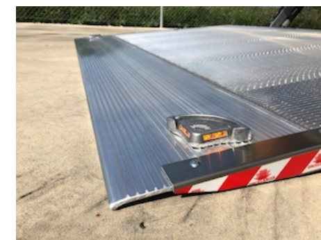
OAE200.B - Flashing platform lights + protection 12/24V
