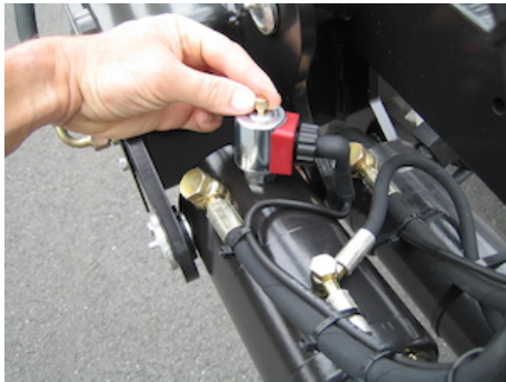
Manual emergency operation on all electrovalves
