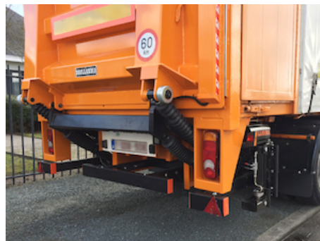
OAF100.ST - Fixed 3-piece bumper in steel, mounted to the lift frame
