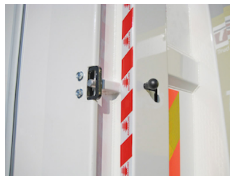
OAP422.L - 1 standard lock on L-side of steel platform
