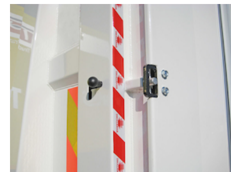
OAP422.R - 1 standard lock on R-side of steel platform
