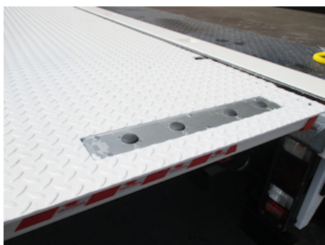
OAE064 - 4-button foot controls + reed sensor in the platform
