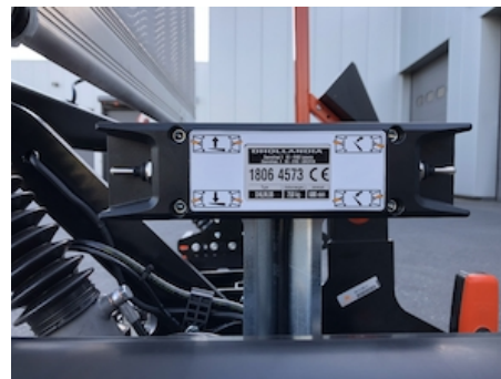
OAE048.0 - Control unit with 2 toggle-switches
