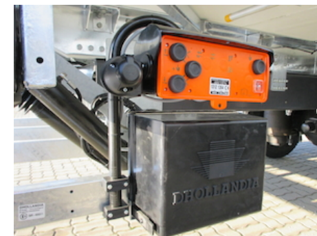
OAM025 - Adjustable mounting bracket for control box
