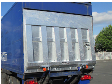
OAT124 - Hot-dip zincplated finish for steel DH-L platform
