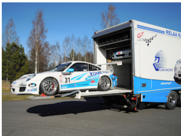
Extended platform with foldable point, for loading & unloading cars, long machines etc...
