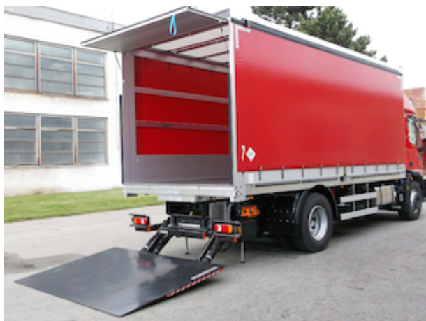
Reinforced heavy-duty steel platform, adapted to extreme lift capacities
