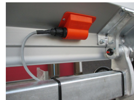
OAE502 - Reed sensor on platform
