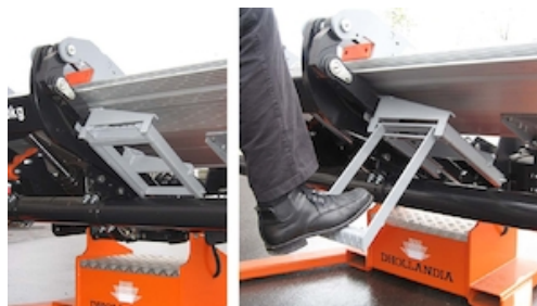
OAM049 - Pull-out foot step mounted on lift arms R...
