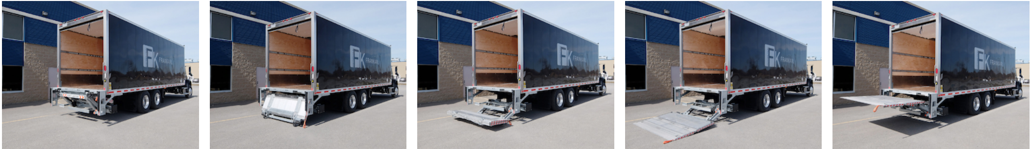
Tail lift with standard bumper bar in 3 sections
