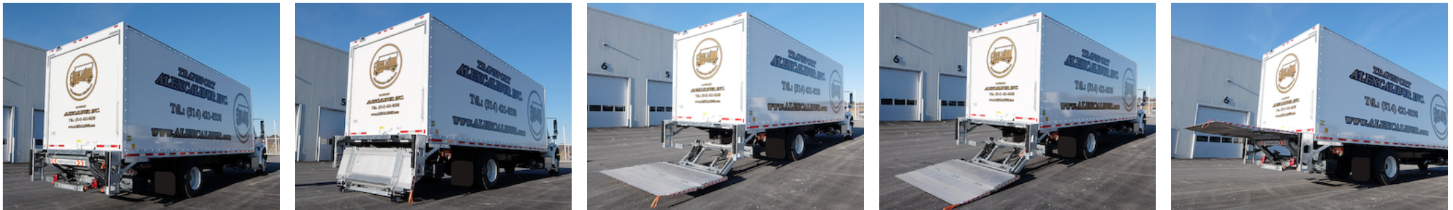
Tail lift with articulated bumper bar for Dock-Lock applications (option)
