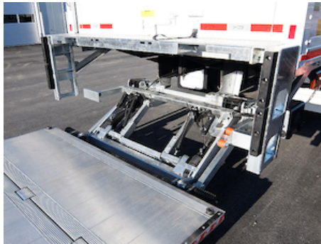
2 lift cylinders for maximum platform stability. Very heavy-duty floor extension plate with height-adjustable side steps and rubber dock buffers
