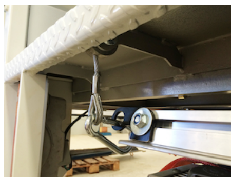
OAP620.C - Platform lock DH-RP with steel cable
