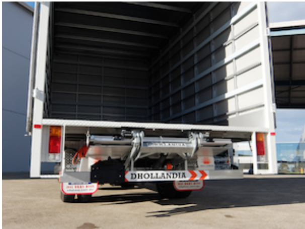
Flush mount with floor plate integrated inside the vehicle body
