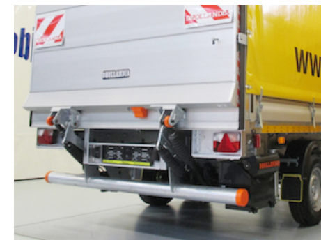
OAF130 - Round bumper tube mounted to the lift arms
