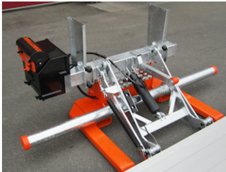
Bolt-on mounting plates for quick and easy fitting [OAM010]
