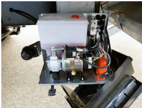
Robust pump unit 12V or 24V DC mounted at the side of the lift frame
