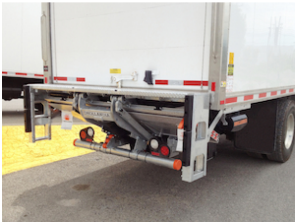
Mounting with floor extension plate added behind the rear sill of the vehicle
