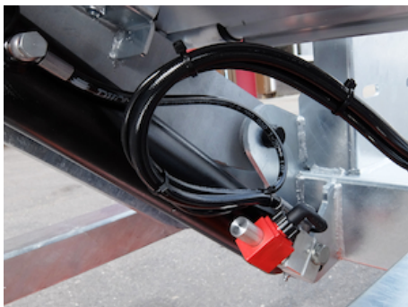
Manual emergency operation on all electrovalves
