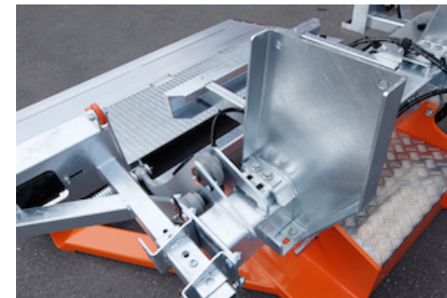
OAM010 - Mounting plates bolted onto lift frame
