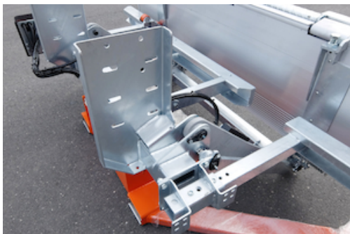
OAM011 - Mounting plates fixed on lift frame
