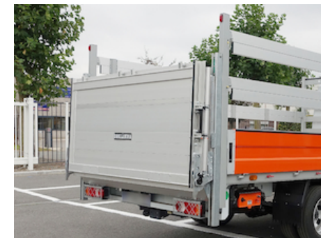
OVT110.1 - Aluminium platform of the DH-VO& K1 / VB& E1 in anodised finish
