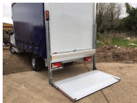
OVP002.0 - Aluminium platform on DH-V* lift
