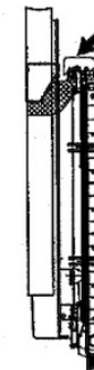
OVP510.A - Shunt stops for vertical descent mounted at the rear edge of the platf
