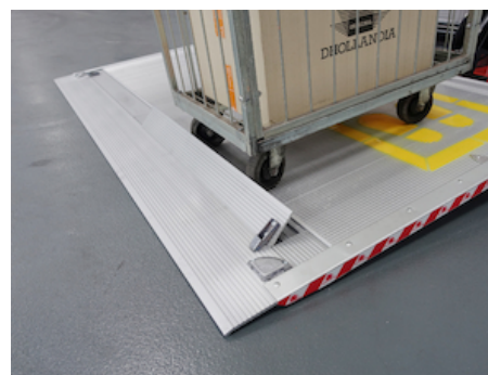
OAP100.M - 2-piece symm. roll-stops in the platform point - MANUAL
