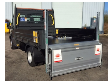
OVP206 - Horizontally foldable platform
