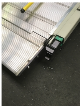
OVP153.400 - Hydr. roll-stops 400 mm + dock supports
