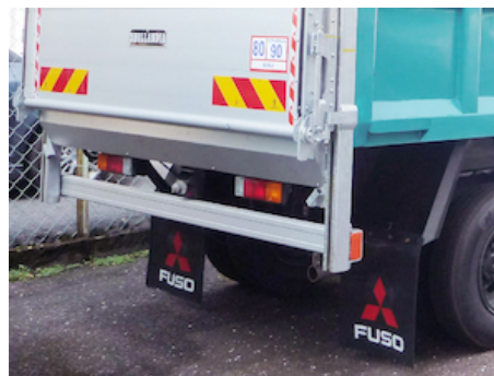
OVF200.A - Aluminium bumper 50 x 100 mm for DH-V*
