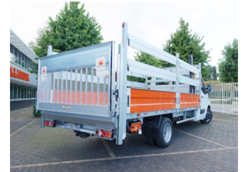
OVP509.A - Permeable platform : alu frame + steel mesh grids
