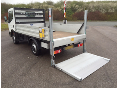
Light-weight aluminium platform with fixed leading edge
