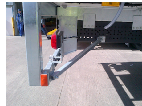
OVF202.01 - Diagonal bumper support for DH-VOxxK1
