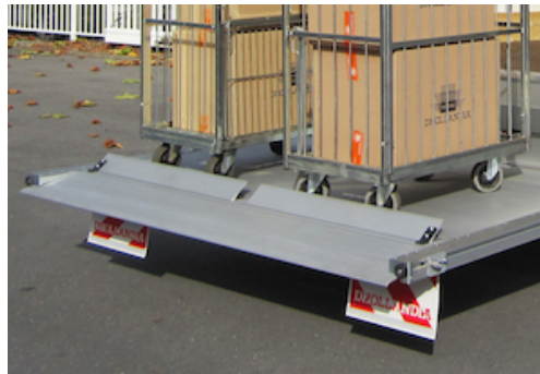
OAP100.M - 2-piece symm. roll-stops in the platform point - MANUAL
