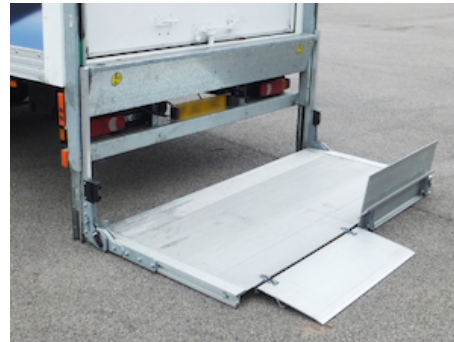
OVP120.A.R - 2 hinged ramps in aluminium at rear edge of platform
