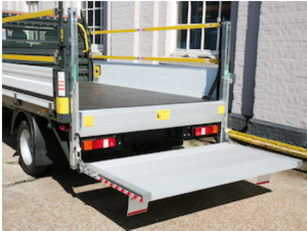
Reinforced lift columns in hot-dip zinc plated steel
