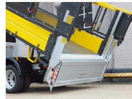
OVU014.A - Dump-over execution type 2 for tipper vehicles
