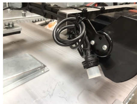
OAE500 - VEHH plug connection for dashboard switch
