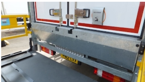
OVF062 - VO.K1 cylinder beam adapted for rear doors
