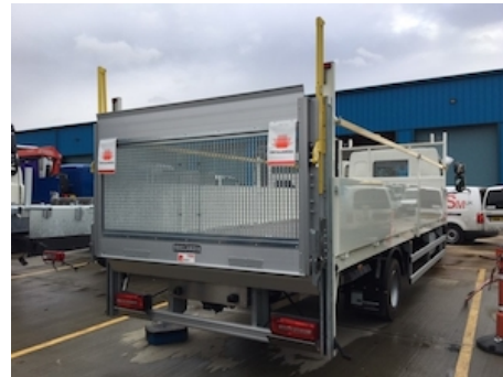
OVP509.G - Open mesh platform + steel grids
