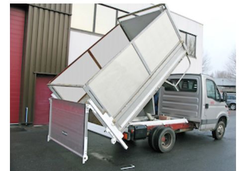
OVU010 - Dump-through execution for DH-VO& K1 on tipper vehicles
