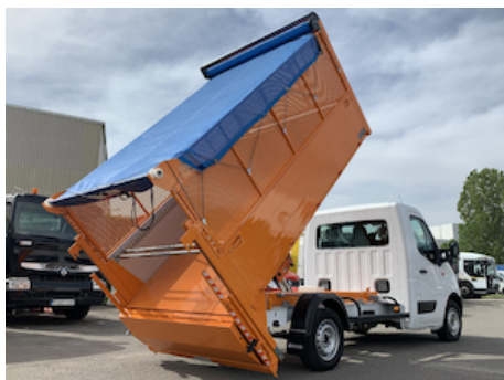
OVU011.S - Dump-over lift T1 for tipper vehicles - steel
