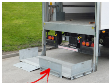
OVP120.S.R - 2 hinged ramps in steel at rear edge of platform
