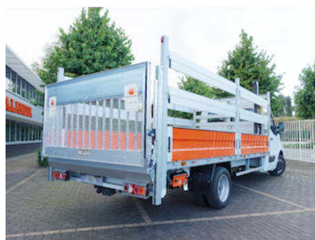
OVP509.A - Permeable platform : alu frame + steel mesh grids
