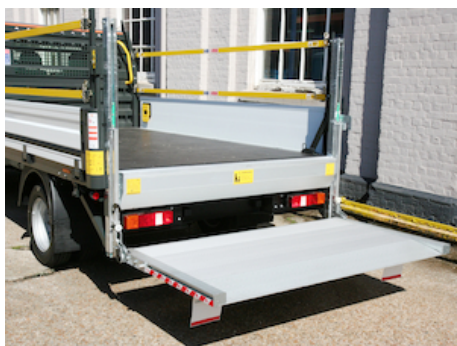
OVT121.F - Lift frame of the DH-VO& K1 / VB& E1 in galvanised finish
