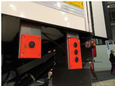
OAM026 - Mounting support type B for OAE031.Z
