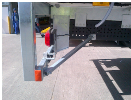
OVF202.01 - Diagonal bumper support for DH-VOxxK1
