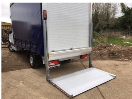
OVP002.0 - Aluminium platform on DH-V* lift
