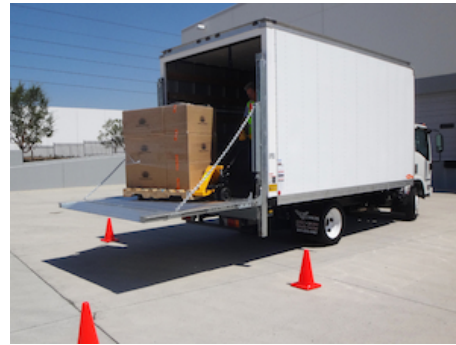
OVU019 - Platform supported by chains
