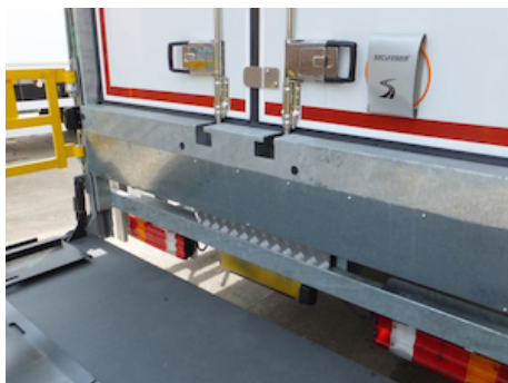
OVF062 - VO.K1 cylinder beam adapted for rear doors
