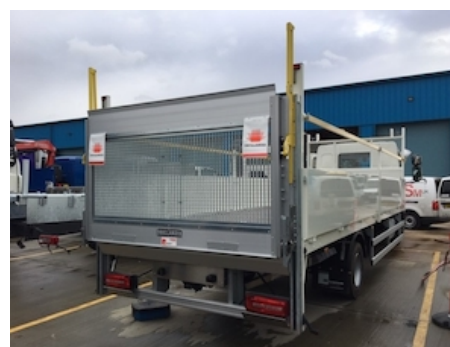
OVP509.G - Open mesh platform + steel grids
