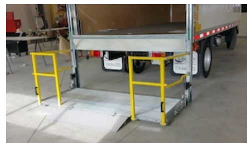
OVU012.A - GAS lift execution of DH-VO& K1 with aluminium platform
