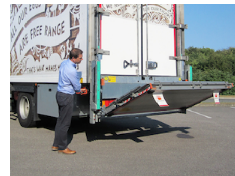
OVH004 - 1 tilt cylinder, no adjustable tilt VOC-VB4
