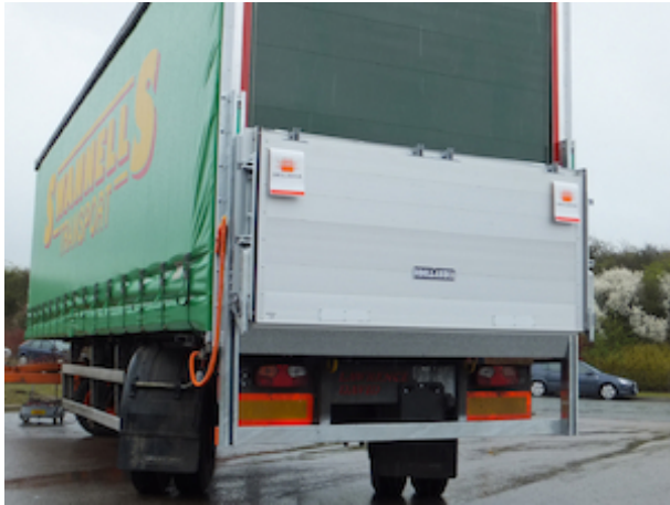
Weight-saving aluminium platform with anti-slip surface
