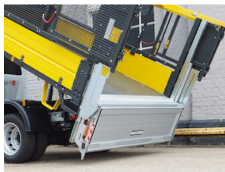
OVU014.A - Dump-over execution type 2 for tipper vehicles
