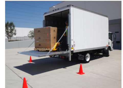
OVU019 - Platform supported by chains
