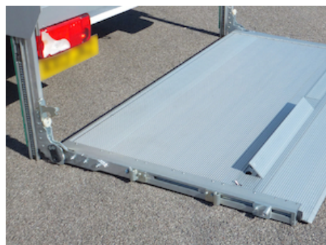
OVP123 - Preparation for demountable side ramp
