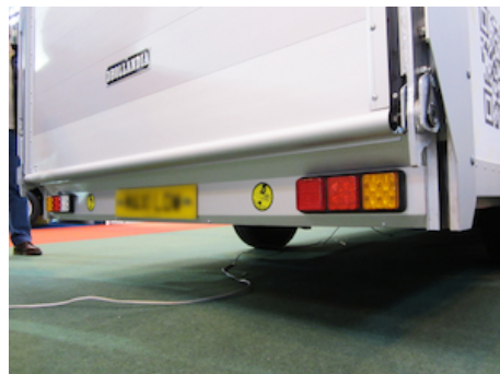
OVF058 - Cylinder beam VO adapted for rear vehicle lights
