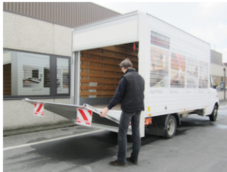
Manual opening and closing of the platform, (where needed) supported by powerful torsion bars
