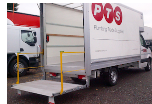
OVP332 - Automatically folding safety rails L+R for DHVO...K1 / VB...E1
