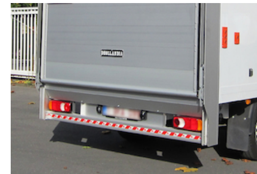
OVF200.A - Aluminium bumper 50 x 100 mm for DH-V*
