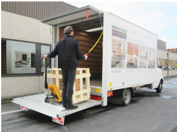
Light-weight aluminium platform with fixed leading edge
