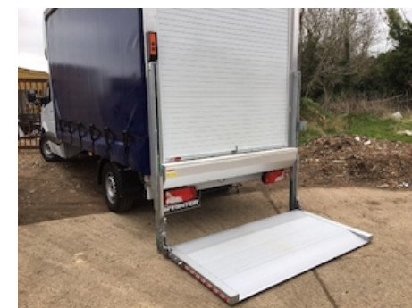
OVP002 - Platform DH-V* manufactured from aluminium
