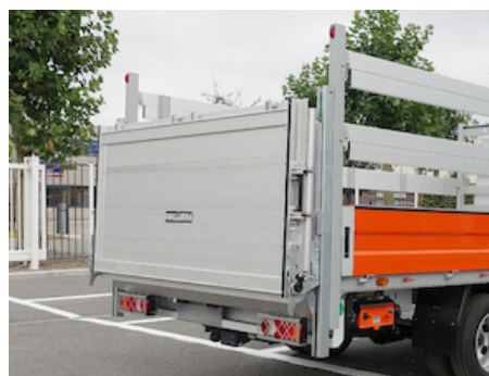
OVT110.1 - Aluminium platform of the DH-VO& K1 / VB& E1 in anodised finish
