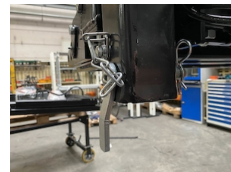
OVF002 - Travel lock pins under the lift runners
