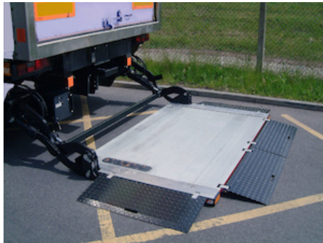
Weight saving aluminium platform with articulated ramps at the outboard edge and the 2 side edges
