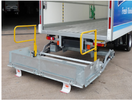
Hot-dip zinc plated steel platform with articulated ramps at the outboard edge and the 2 side edges
