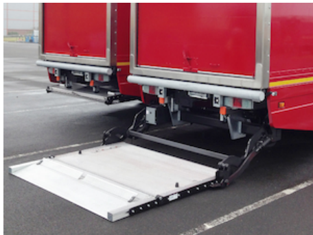
Foldable platform with fixed leading edge, installation in shorter overhang (mounting space)
