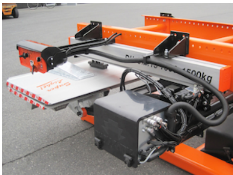
Robust pump unit 12V or 24V DC mounted at the side of the lift frame
