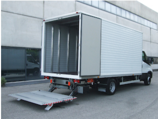
Weight-saving full aluminium platform (base section + foldable point)
