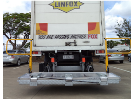
OAP204.LR - 2 hinged safety rails with rotating foot on L+R side of platform
