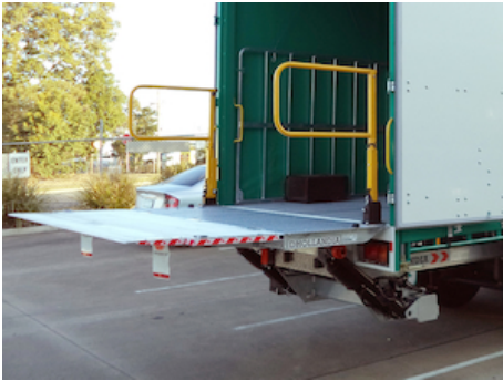
OAP203.LR - 2 hinged safety rails on L+R side of a foldable platform
