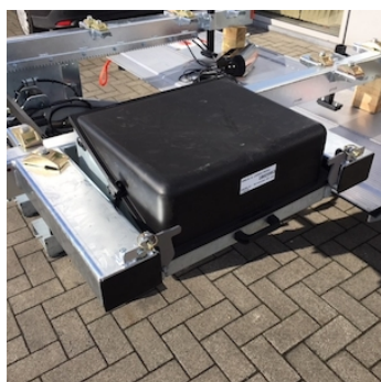
OAE406.24.TL - 24V battery box on slide tubes - telescopic
