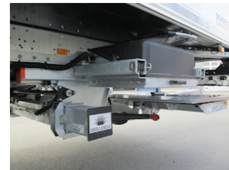
OAE406.24.L - 24V battery box on slide tube low
