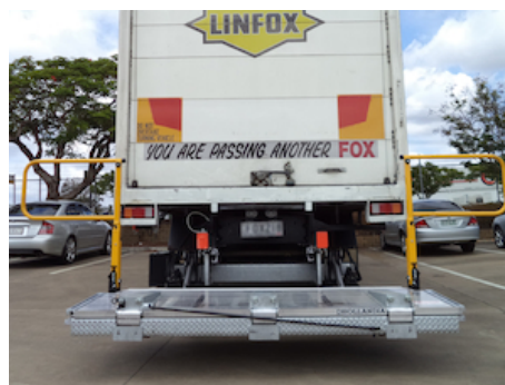
OAP204.LR - 2 hinged safety rails with rotating foot on L+R side of platform
