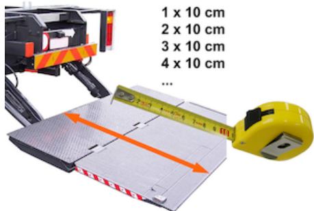
OAP602 - Extension of the slider lift platform per 10 cm
