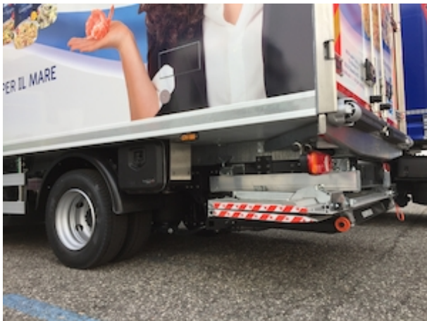
Compact lift frame and a double-folded platform for mounting in a very short mounting space
