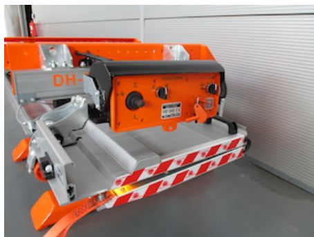
Electrical controls without sensitive electronic components
